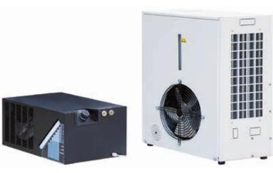
AWEX air/water heat exchangers are the ideal solution for water cooling in applications which do not require operating temperatures lower than the ambient temperature (cooling of spindles, cooling of welding...). The heat exchange occurs between the ambient air and the fluid that is conveyed into the exchanger and it is cooled by the fan-forced air. The main advantages of the AWEX range are reduced dimensions, a good quality/price relationship and easy maintenance.
