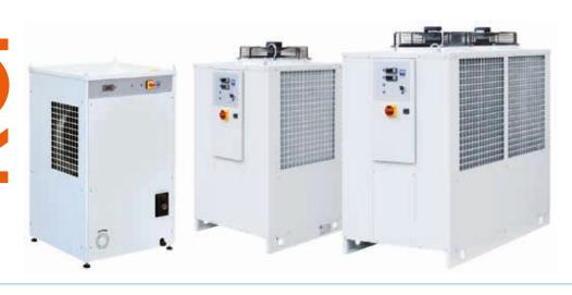
RCF-SD is a new series of Euro Cold coolers designed to cool cutting fluids, cooling and lubricating fluids that contain impurities, even though they have been filtered. Careful design and experimentation allowed us to deploy an innovative solution thanks to a special evaporator: thanks to a wide cross-section, it can cool with direct exchange of the fluid through a cooling gas.
